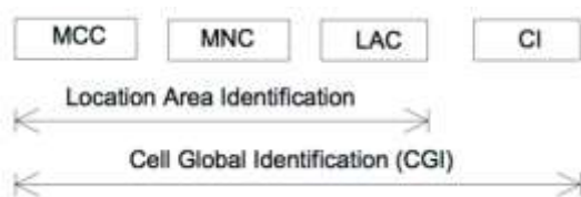
Figure 3.3 Comparison of location area identification (LAI) and cell global identification (CGI) Source: ETSI TS 123 003
